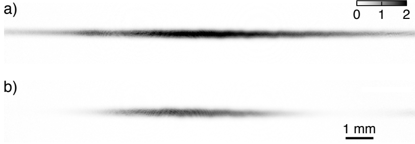
Figure 3.9: Absorption image of the atomic ensemble after release from the dipole trap and 1 ms time-of-flight. a) Fully loaded dipole trap with 20 M atoms. b) Reduced ensemble with 9 M atoms. The greyscale denotes optical density.
