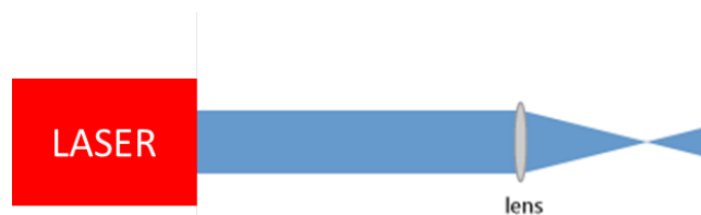
Figure 1.1: A laser beam can be well collimated and focused to diffraction-limited spot sizes.
