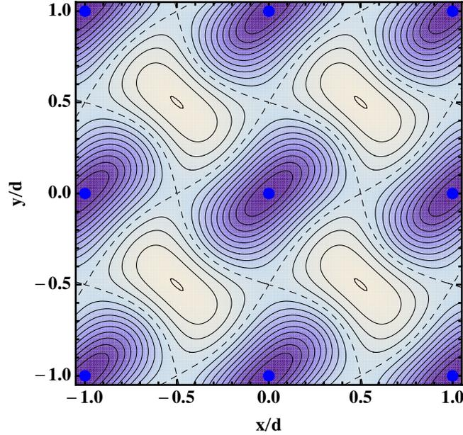
**Figure 2.** Zeeman pseudo-potential (equation (12)) in the trapping plane ( $z = h = d/2$ ) produced by the magnetization pattern of figure 1 at a Ioffe field strength that creates equal potential barriers (dashed separatrix) between the potential wells (blue points) in the two lattice directions (16). Darker colors signify deeper potentials.
