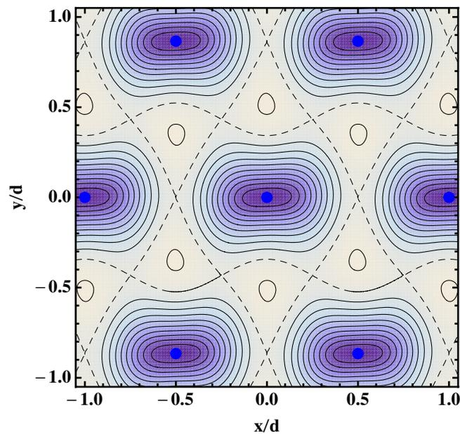
**Figure 4.** Zeeman pseudo-potential (equation (12)) in the trapping plane ( $z = h = d/2$ ) produced by the magnetization pattern of figure 3 at an Ioffe field strength which creates equal potential barriers (dashed separatrix) between the potential wells (blue points) in the three lattice directions (16). Darker colors signify deeper potentials.
