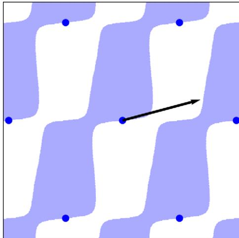
**Figure 3.** Optimized magnetization pattern for a triangular lattice of IP traps (above blue points) constrained by equation (17) with  $\psi = 5\pi/12$  and additional field constraints at the potential barrier given in the text. The nominal trapping height is  $h = d/2$ , and the Ioffe direction is indicated by the arrow. The optimization yields  $C = 0.729$ . Blue (white) areas are fully magnetized (unmagnetized) with  $m = 1$  ( $m = 0$ ).
