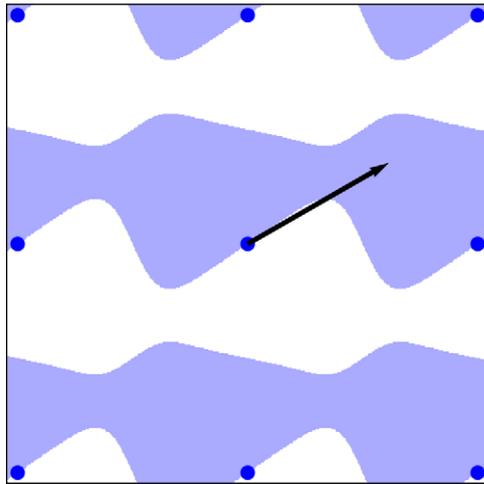
**Figure 1.** Optimized magnetization pattern for a square lattice of IP traps (above blue points) constrained by equation (17). Trapping height is  $h = d/2$ , and the Ioffe direction is given by the arrow ( $\psi = \pi/3$ ). The optimization yields  $C = 1.06$  in equation (17). Blue (white) areas are fully magnetized (unmagnetized) with  $m = 1$  ( $m = 0$ ).
