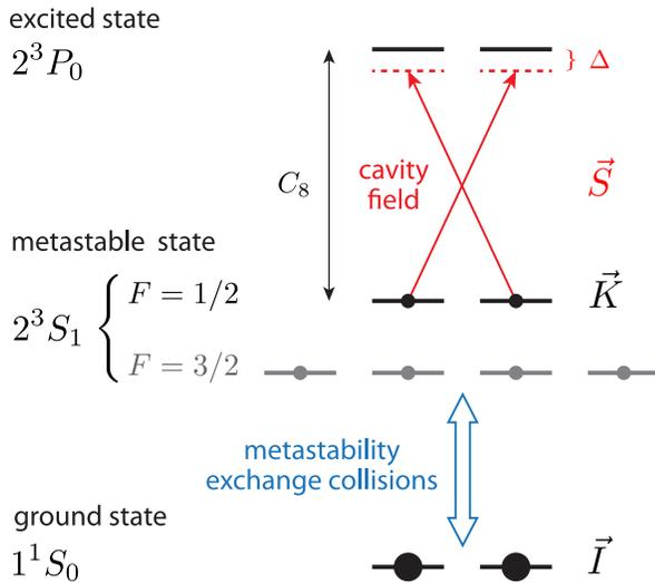
FIG. 2. Relevant level scheme of  ${}^3\text{He}$  for  $z$  quantization axis, which corresponds to the cavity axis. The cavity mode (red) addresses the  $C_8$  transition between the  $F = 1/2$  metastable manifold and the  $F = 1/2$  excited state  $2^3P_0$ , with detuning  $\Delta$ . The six metastable levels  $2^3S_1$  are coupled to the purely nuclear  $1^1S_0$  ground state by metastability exchange collisions.
