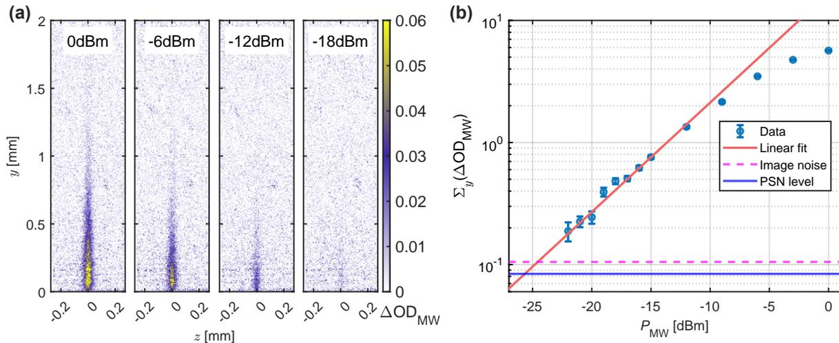
FIG. 4: (a) Images of  $\Delta OD_{MW}$  for single-tone MW signals of different power  $P_{MW}$ . Here,  $\tau_{MW} = 2 \mu s$  and other conditions are as in Fig. 2(a). (b) Peak values of the Gaussian fit to the integrated spectrum  $\Sigma_y(\Delta OD_{MW})$  with  $y \in [0, 1.2 \text{ mm}]$ , as a function of  $P_{MW}$ . The linear fit is performed on the leftmost 9 points, the magenta dashed line is the noise level without MW, and the blue solid line is the photon shot noise level.
