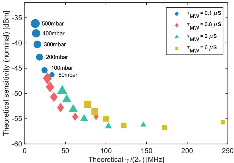
FIG. 7: Theoretical dependence of the FWHM frequency resolution and the nominal MW power sensitivity on the MW pulse length and buffer gas pressure. The nominal MW power sensitivity is estimated for the current MW setup and normalized to 1 s integration time.
