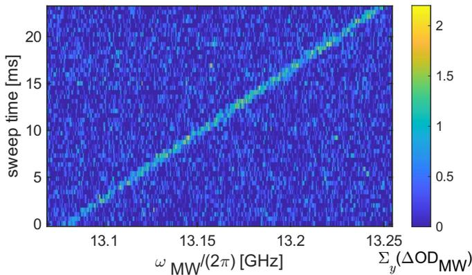
FIG. 6: Spectrogram of frequency-swept MW signal. Each line represents the integrated signal  $\Sigma_y(\Delta\text{OD}_{\text{MW}})$  over the selected 20-row-image measured within 480  $\mu\text{s}$ . With 50 measurements during the 24 ms sweep time, all timings are confirmed by a separate oscilloscope triggered by the camera exposure pulse. The measurement confirms the linearity of the MW frequency sweeping process.
