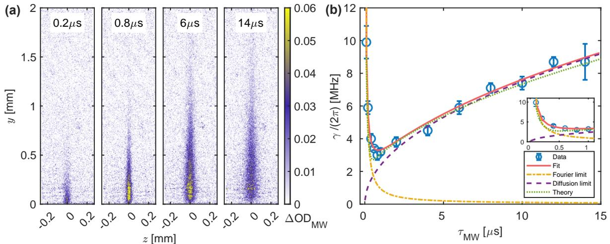
FIG. 3: (a) Images of  $\Delta\text{OD}_{\text{MW}}$  for different  $\tau_{\text{MW}}$  and other conditions as in Fig. 2(a). (b) Signal width  $\gamma$  as a function of  $\tau_{\text{MW}}$ . Red solid line: fit (see text); yellow dash-dotted line: Fourier limit and intrinsic linewidth  $\gamma_0$ ; purple dashed line: diffusion limit; green dotted line: simulation result. Inset: zoom into the region  $\tau_{\text{MW}} < 1 \mu\text{s}$ .
