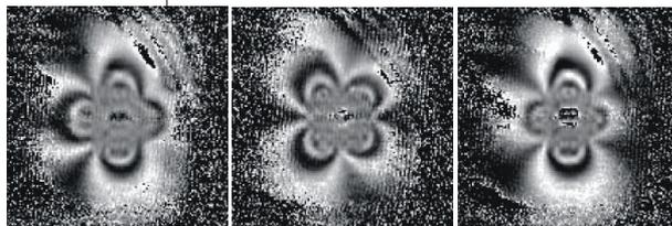
sensitive to the circuit geometry and electric current distributions, both of which may often be complex. In this context, Böhi *et al.* have used a cloud of cold rubidium atoms to characterize and map out the magnetic component of a microwave circuit. The atoms are prepared in an initial state sensitive to local magnetic fields. As the atoms sense the effect of the magnetic field generated in the circuit, they drop out of their initial state. Absorption imaging with a laser beam can then
